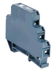
configuration is made of a two stage cascade, using Gas Discharge Tube - GDT and Silicon Avalanche Diode - SAD technologies, coordinated through a series impedance, giving an effective and extremely fast protection.
